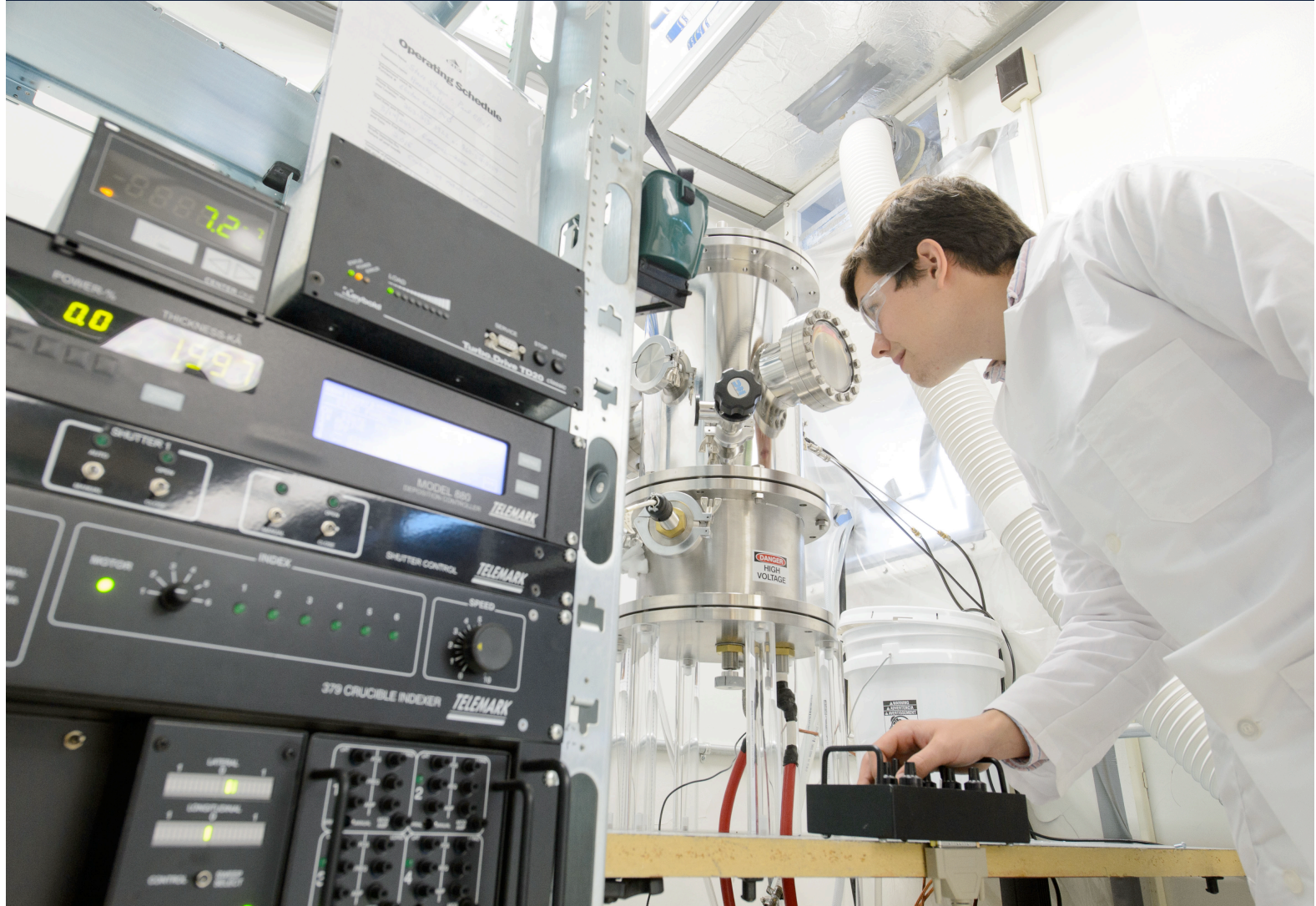
S. Stagon; doctoral student of mechanical engineering, with nanorod growing apparatus at the Longley Building (Peter Morenus/UConn Photo)
